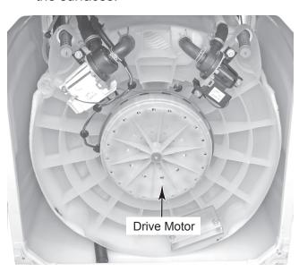
6. Use a 1/4" Allen wrench and loosen the rotor mounting screw as far as it will go (the screw is captive and cannot be removed from the rotor). The rotor is seated on the splined tub shaft. Rock the rotor back and forth and pull it off the shaft so it contacts the screw washer-head, then further loosen the screw. Do this until the rotor is removed from the shaft.
