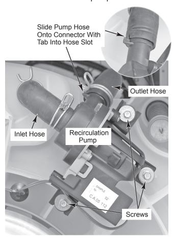
c) Disconnect the 2-wire connector from the recirculation pump terminals.
