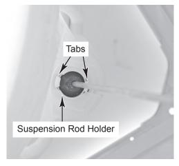
d) Position the suspension rod through the slot in the tub opening, and remove the rod assembly from the washer.
