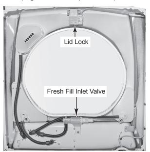
b) Loosen the clamp and disconnect the end of the fresh fill inlet valve hose from its water inlet/dispenser valve connector (see the top right photo). NOTE: The fresh fill inlet valve hose is permanently attached to the inlet. It is not intended to be removed.  Remove the screw from the fresh fill inlet valve and remove the valve assembly.
