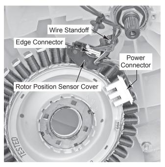
12. Pry up on the two locking tabs and pull the rotor position sensor cover off the stator housing. **NOTE:** In the top right photo, there are two indents on the housing to mark where the rotor position sensor cover is installed. Be sure to snap the two tabs on the rotor position sensor cover into these indents when you reinstall it on the stator assembly.
