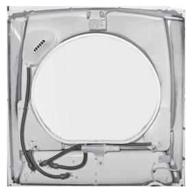
Loosen the clamps and remove the four hoses going to the water inlet/dispenser valve assembly.
