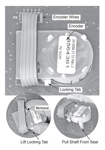
**NOTE:** Before you can remove the user interface board, you must first remove the encoder.
