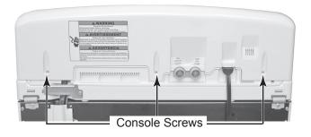
Lift the console off the cabinet and disconnect the user interface board cable connector at machine/motor control connector P11.
