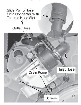
c) Open the wire cover on the pump and disconnect the 2-wire connector from the terminals.
