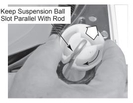
c) Reach down along the side of the tub, and press in on the suspension rod holder locking tabs, then push the holder out of the tub opening.
