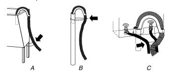
If the washer faucets and the drain standpipe are recessed, put the formed end of the drain hose into the standpipe. Tightly wrap the tie strap around the water inlet hoses and the drain hose. See view C.
