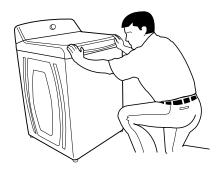
Lower right front foot until it contacts the floor. By hand, firmly rotate foot as much as an additional 1-1/2 turns. The other three feet have been preset at the factory.
