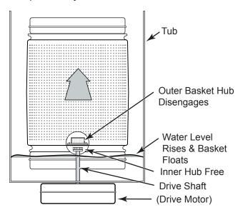
When the tub drains, the basket drops back to it's original position, and the hub components re-engage, connecting the basket to the shaft, and permitting the basket to spin.
