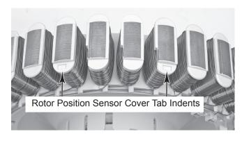
REASSEMBLY NOTE: When you reinstall the drive motor rotor over the stator assembly, do not grip the rotor housing around the rear edge with your fingers. The magnets around the rotor housing are very strong, and they will pull the rotor into the stator coil magnets when the rotor magnets come within their magnetic field. Keep your fingers along the outside of the rotor housing and away from the rear edge when you are installing it on the stator assembly.
