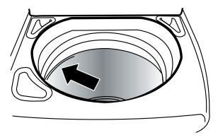
Pour measured powdered or liquid High Efficiency (HE) detergent into the detergent dispenser. Do not put detergent directly into the wash tub or onto clothes in the washer.
